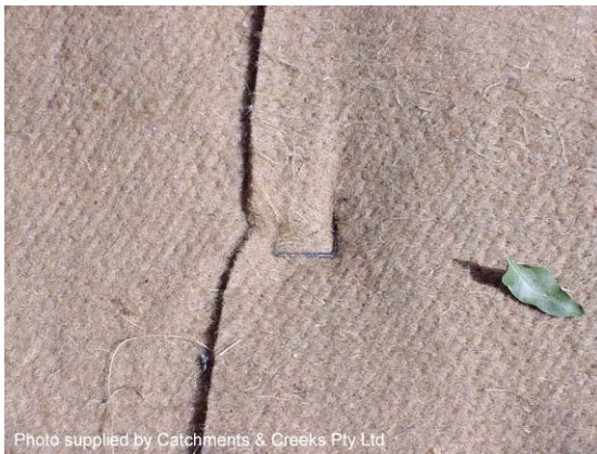
Photo 3 – Jute blanket (thick)
