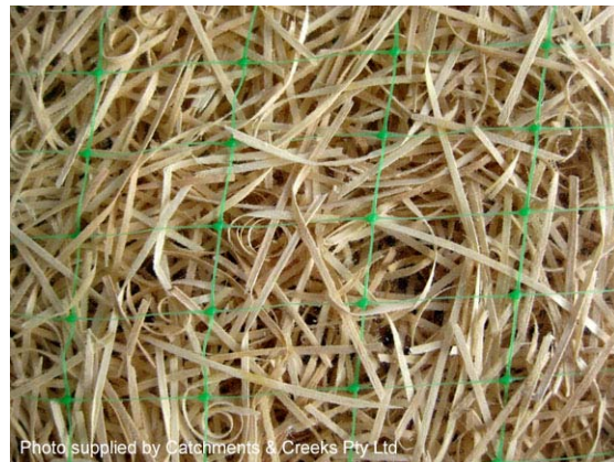
Photo 4 – Wood shaving blanket with temporary synthetic netting
