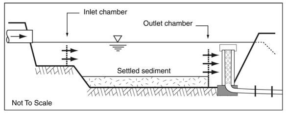
Figure 8 – Typical arrangement of outlet chamber (long section)
