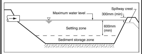
Figure 4 - Settling zone and sediment storage zone
