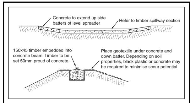
Figure 12 - Typical detail for a Type A and B basin level spreader
