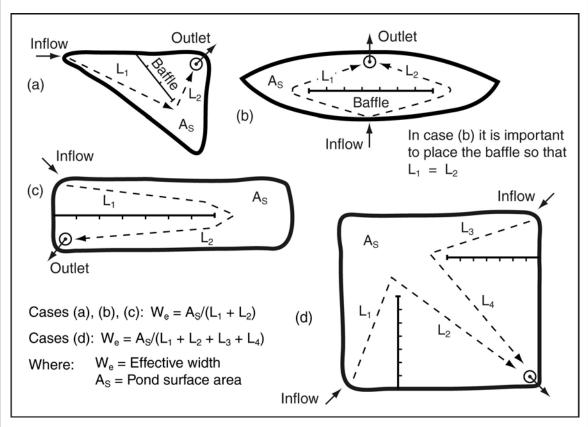
Figure 6 – Typical arrangement of internal flow control baffles (after USDA, 1975)
