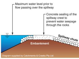
Figure 21 - Sealing of spillway crest
