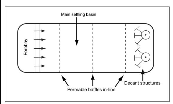
Figure 7 – Typical arrangement of in-line permeable baffles
