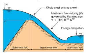
Figure 20 - Basin spillway hydraulics
