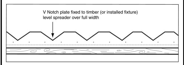
Figure 13 – Typical detail for multiple V-notch weir plate
