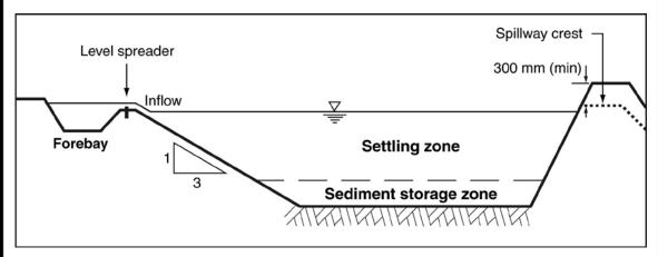
Figure 2 - Long-section of a typical Type B basin
