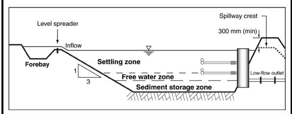
Figure 1 – Long-section of a typical Type A basin
