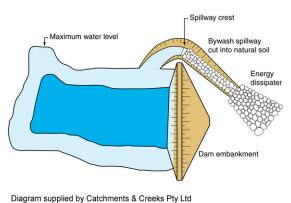
Figure 22 – Spillway cut into virgin soil
